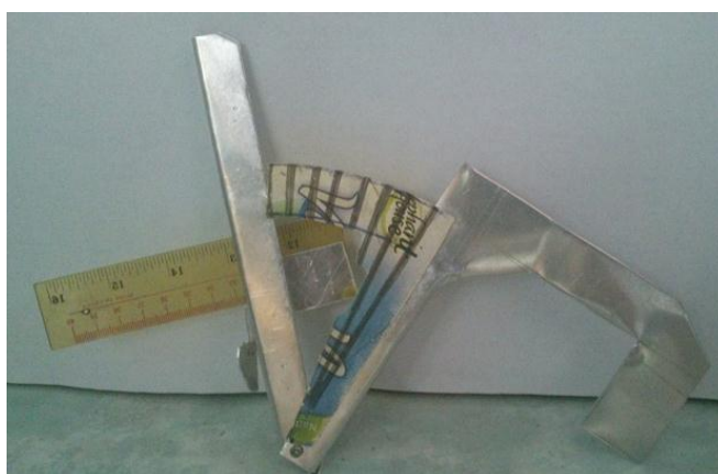
Figure 11 - Equipment to measure stiffness of tea shoots
