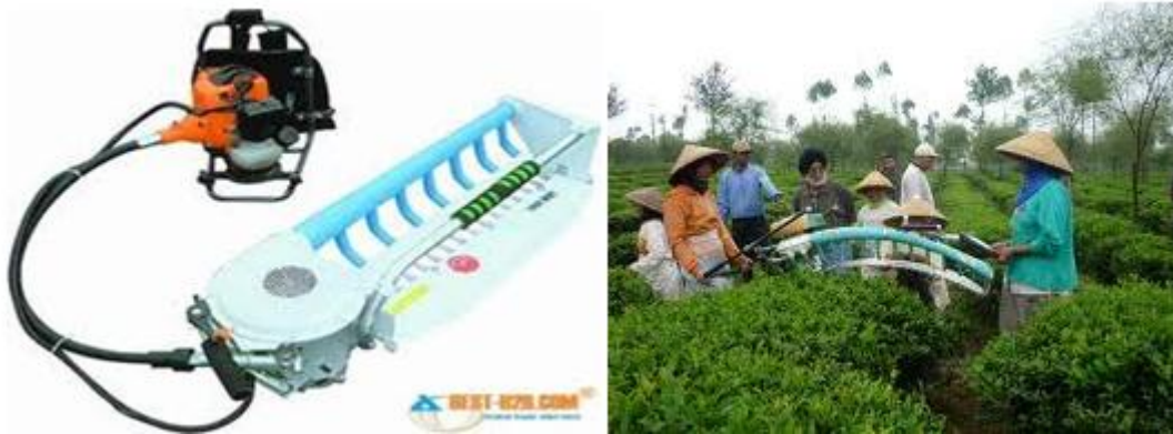
Figure 9: Machines with reciprocating cutters (source: [42])
