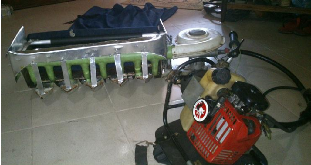
Figure 31 - Tea harvester machine with the attachment
